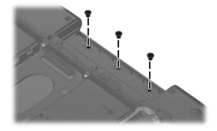
5. Remove the three Phillips PM2.0×3.0 screws in the optical drive bay.
